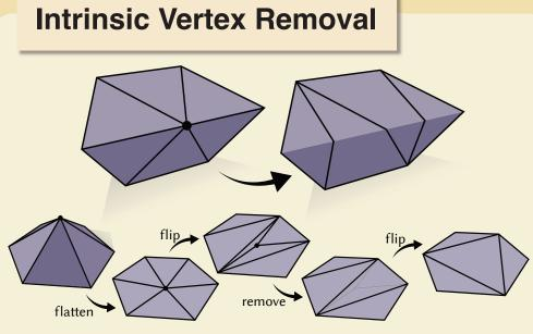
We decimate an interior vertex by intrinsically flattening it, flipping to degree 3, removing it from the mesh, then flipping back to an intrinsic Delaunay triangula-
