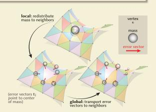
Our method constructs a coarse triangulation over a fixed geometric domain. In each **local** step we redistribute curvature or other quantities from a removed vertex to its neighbors. From step to step we also accumulate global information about error via tangent vectors pointing to the approximate center of mass of the decimated vertices.
