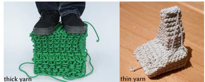
Fig. 24. Changing the yarn material changes the properties of solid-knit objects. Here we show two hand-knit examples. Using a thicker yarn can create sturdy objects quickly, but the results will be lower resolution ( left ). Conversely, using thinner yarn can create higher resolution objects but takes significantly longer ( right ).
